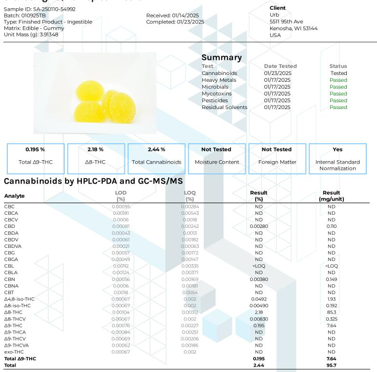
ND = Not Detected; NT = Not Tested; LOD = Limit of Detection; LOQ = Limit of Quantitation; RL = Reporting Limit;  $\Delta$  = Delta; Total  $\Delta$ 9-THC =  $\Delta$ 9-THC \* 0.877 +  $\Delta$ 9-THC; Total CBD = CBDA \* 0.877 + CBD;
